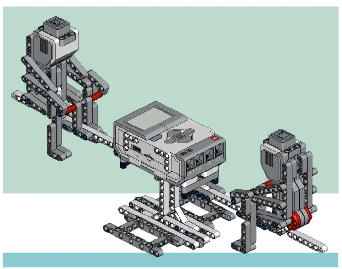
This model is made of LEGO® MINDSTORMS<sup>™</sup> 45544 core set & 45560 expansion set
