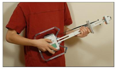
Hold the sliding plate with your left hand with your hand on the side away from the ultrasonic sensor. Slide the plate up and down the guitar's neck to select the note to play, then press the orange button on the NXT with your right thumb to play the note.
