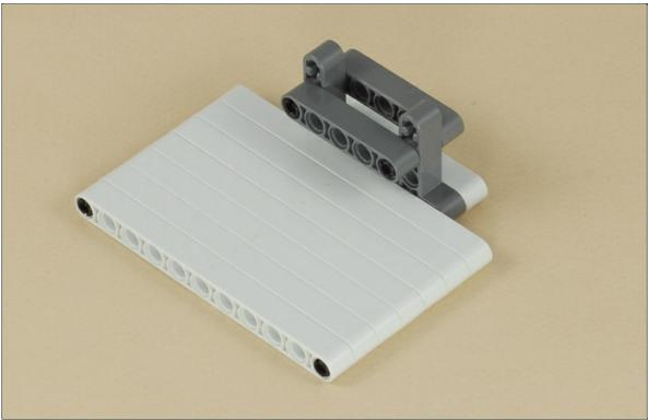
The ultrasonic sensor needs something hard and flat to measure distance to, so that is what this sliding plate is for. The ultrasonic sensor does not work when something is too close to it, so the two pegs sticking out of the neck near the sensor prevent the plate from getting closer than about  ${\bf 1}$  inch from the sensor.
