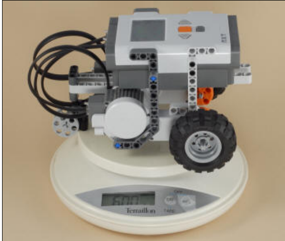
The Castor Bot's total weight is 600 grams
