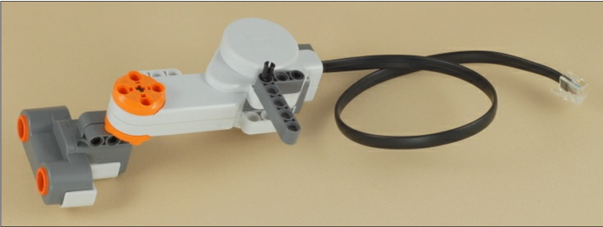
Connect the wire from the "neck" motor to port A on the NXT.
