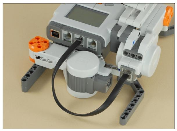
Connect the medium-length wire from the second (tail) motor to port  ${\bf C}$  on the NXT.
