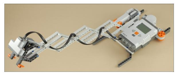
Connect the shortest wire from the neck motor to port  $\boldsymbol{\mathsf{B}}$  on the NXT.
